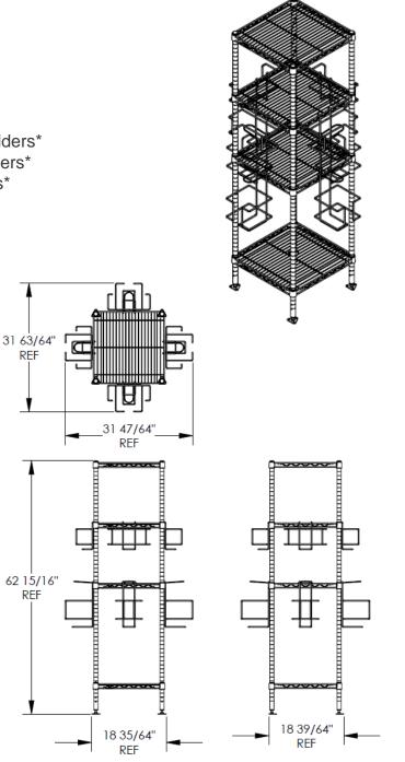
Unit Weighs: 43lbs NSF Components and ADA Compliant
